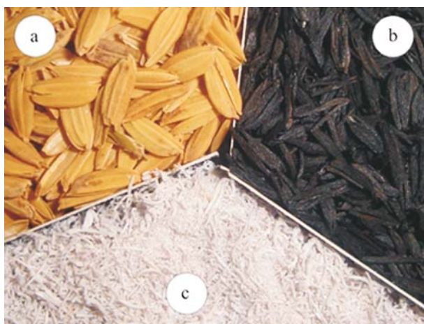
Fig. 1 Appearance of ungrounded a – RRH, b – BRHA and c – WRHA
